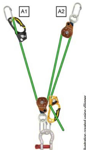
As expected, the results indicated that Anchor Point One (A1) received 1/3 of the applied force and Anchor Point Two (A2) received 2/3 of the force. These control tests confirmed well-established pulley systems principles and also created a baseline for comparison to the user-configured test examinations.
