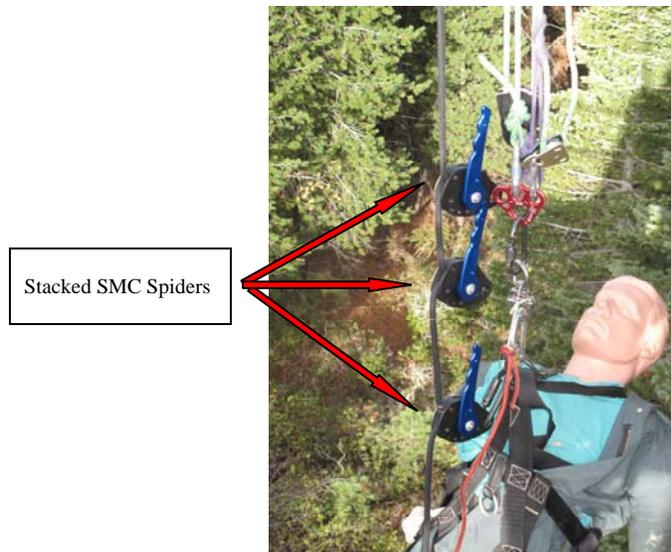
Stacked drop test set-up
