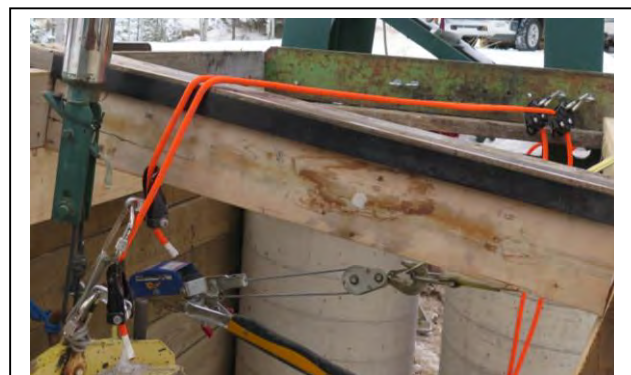
Offset Mass Sharp Edge Test, Ropes Held by Rope Grabs
