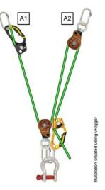
As expected, the results indicated that Anchor Point One (A1) received 1/3 of the applied force and Anchor Point Two (A2) received 2/3 of the force. These control tests confirmed well-established pulley systems principles and also created a baseline for comparison to the user-configured test examinations.
