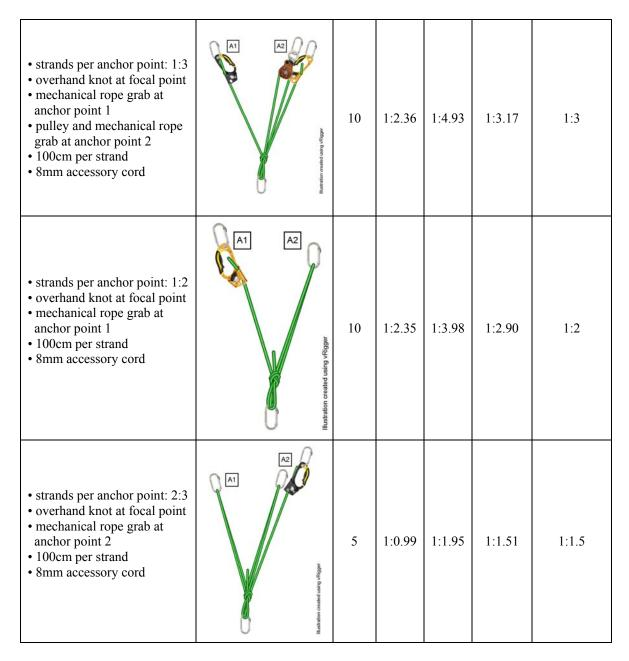
We began our examination of field replicable anchor system configurations by initially focusing on test setups that included an equal number of strands per anchor leg. Figure 6 summarizes statistics for both '1 strand vs. 1 strand' and '2 strands vs. 2 strands' (1:1 and 2:2) using Short R.I.S.
